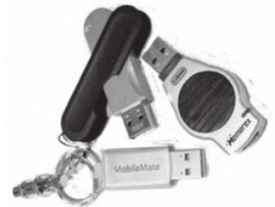
Figure 3.17 Solid-state storage devices have a variety of names. Memory stick, thumb drive, and travel disk are commonly used. The standard name is USB flash drive or “UFD.”
