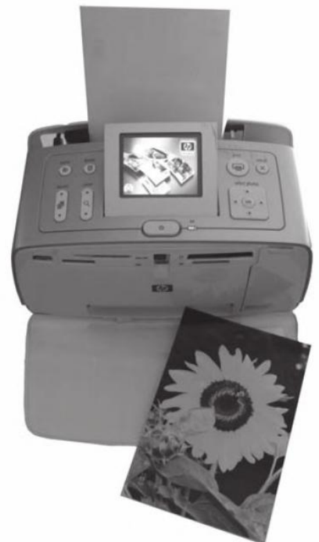
Figure 3.27 Photo printers can crop, enlarge, and enhance the image before printing on special photo paper.
