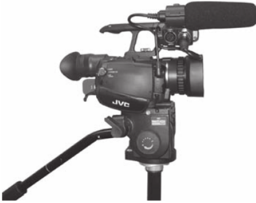
Figure 8.1 Digital video camera considerations include quality of CCDs, lenses, and microphone; storage type and capacity; and light sensitivity.
