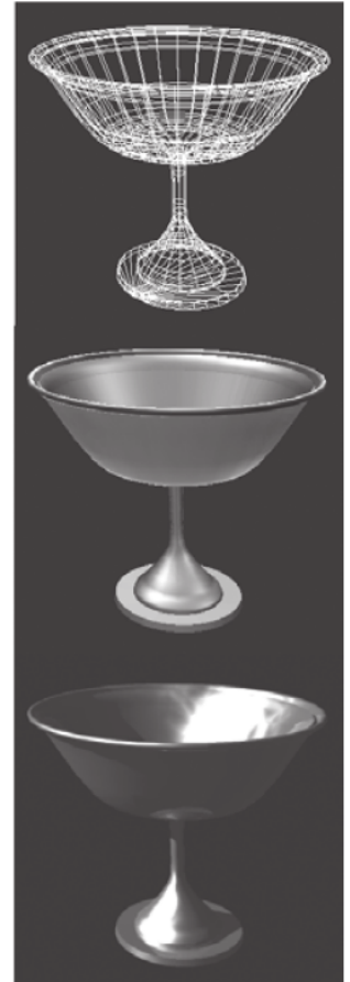
Figure 6.35 Rendering options: wire frame (top), smooth shading (middle) and ray tracing (bottom). See Color Plate 22.
