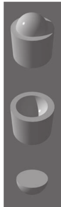
Figure 6.27 Boolean CSG: union (top), difference (center), intersection (bottom). See Color Plate 17.
